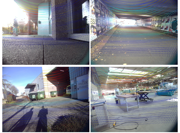
Figure 3. Example camera images overlaid with projected LiDAR points, colored by depth. Top: Stadtgarten scene near building (left) and the GNSS-denied underpass tunnel (right). Bottom: Construction Hall scene entrance area (left) and the indoor construction hall (right).
